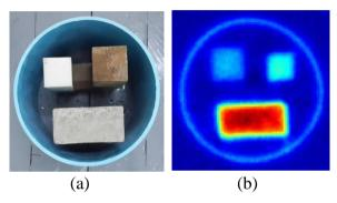
Figure 9 The comparison of(a) the optical camera image and (b) the reconstructed crosssectional image of the interior density distribution of different density objects
