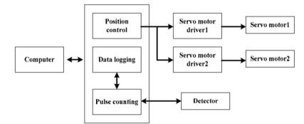
Figure 6 The block diagram of the operation of the CT system
