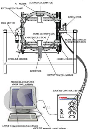
Figure 3 General arrangement of whole GORBIT system
