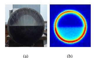
Figure 11The comparison of (a) the optical camera image and (b) the reconstructed crosssectional image of the phase distribution in the pipe
