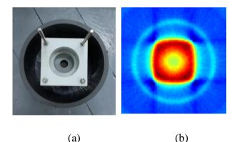
Figure 10The comparison of (a) the optical camera image and (b) the reconstructed crosssectional image of the internal structure of the lead block
