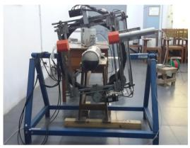
**Figure 5** The vertical arrangement for the measurement of the phase distributionin the pipe
